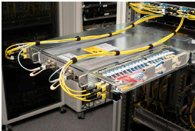
**Figure 5:** HDEA in Service with Side Cover Removed, Exposing 40 of the 80 10G Optics
