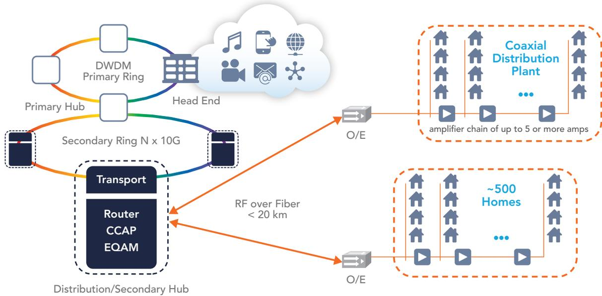
Figure 1: A Typical Pre-DAA HFC-based Cable Access Network
