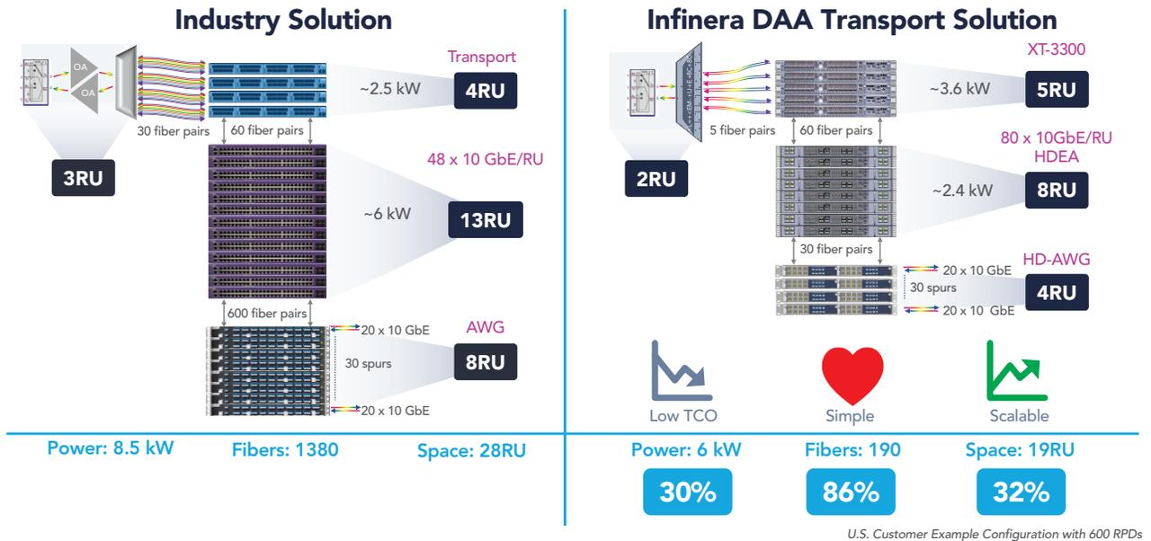
Figure 6: Space and Fiber Savings from Infinera’s DAA Transport Solution
