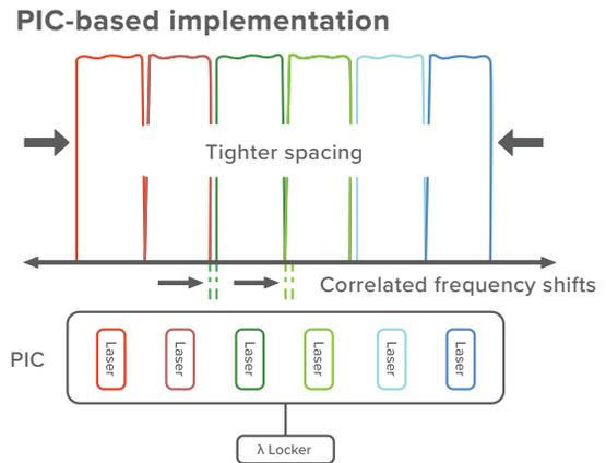
**Figure 6b:** Six-carrier large-scale PIC implementation with single wavelocker
