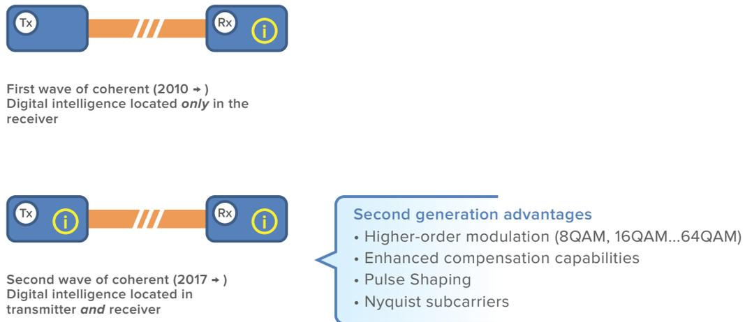
**Figure 1:** The first and second waves of coherent processing
