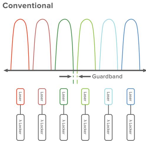
**Figure 6a:** Conventional transponders use separate wavelockers
