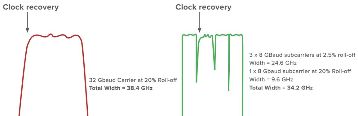
**Figure 5:** Roll-off reduction using inner subcarrier coherent clock recovery
