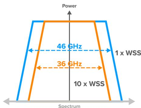
FIGURE 6: Filter narrowing and WSS cascades
