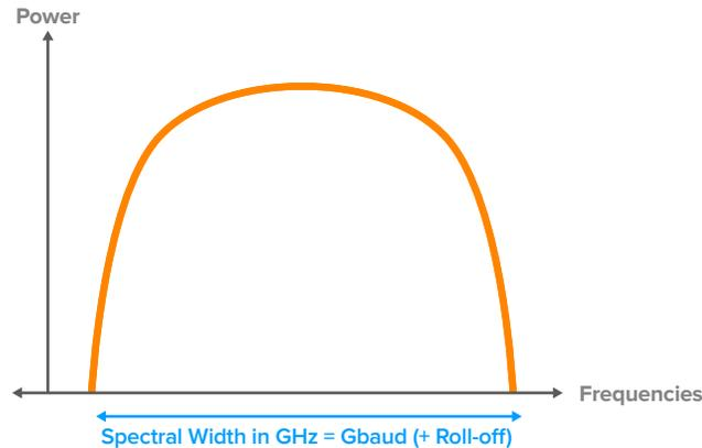
*FIGURE 1: Spectral width is proportional to baud rate*
