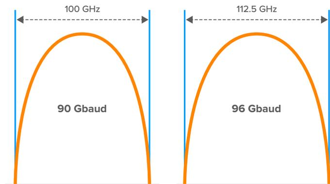
*FIGURE 9: Simplified Flexible-grid Operations with 90 Gbaud and 100 GHz*
