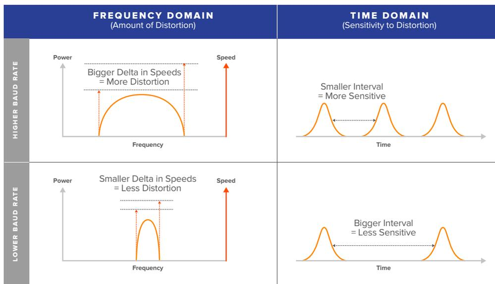
FIGURE 5: Higher baud rates and chromatic dispersion
