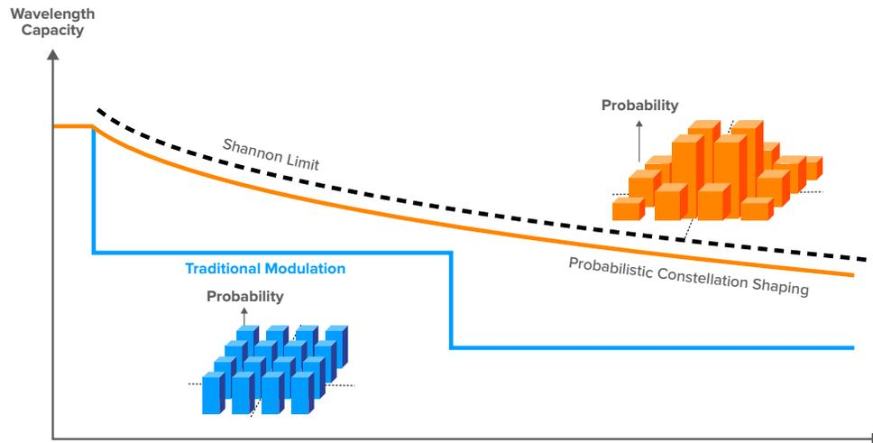
FIGURE 3: Probabilistic constellation shaping
