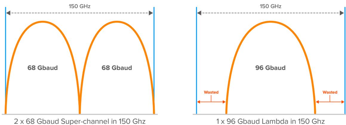
**FIGURE 8:** Lower baud rates can align better with available spectrum
