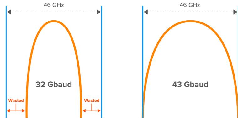
**FIGURE 7:** 50 GHz Fixed-grid point-to-point is limited to ~43 Gbaud
