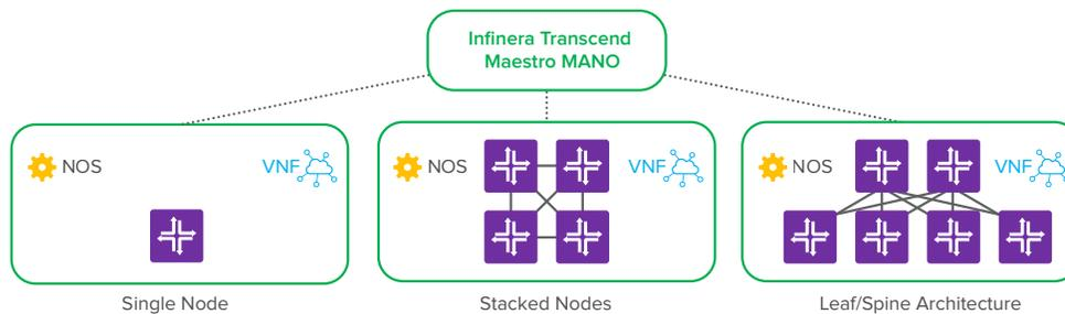
Figure 2: Highly Scalable Network Element Architecture Options
