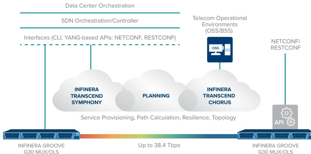
Figure 2: Groove G30 MUX Management and Control
