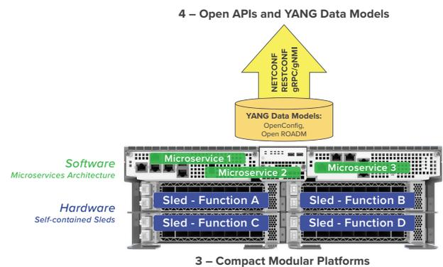
Figure 2: Open optical networking requirements 3 (compact modular) and 4 (open APIs/YANG)
