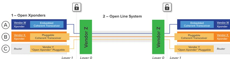
Figure 1: Open optical networking requirements 1 (open Xponders) and 2 (open line system)
