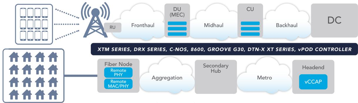
Figure 2: Infinera Solutions for 5G and DAA
