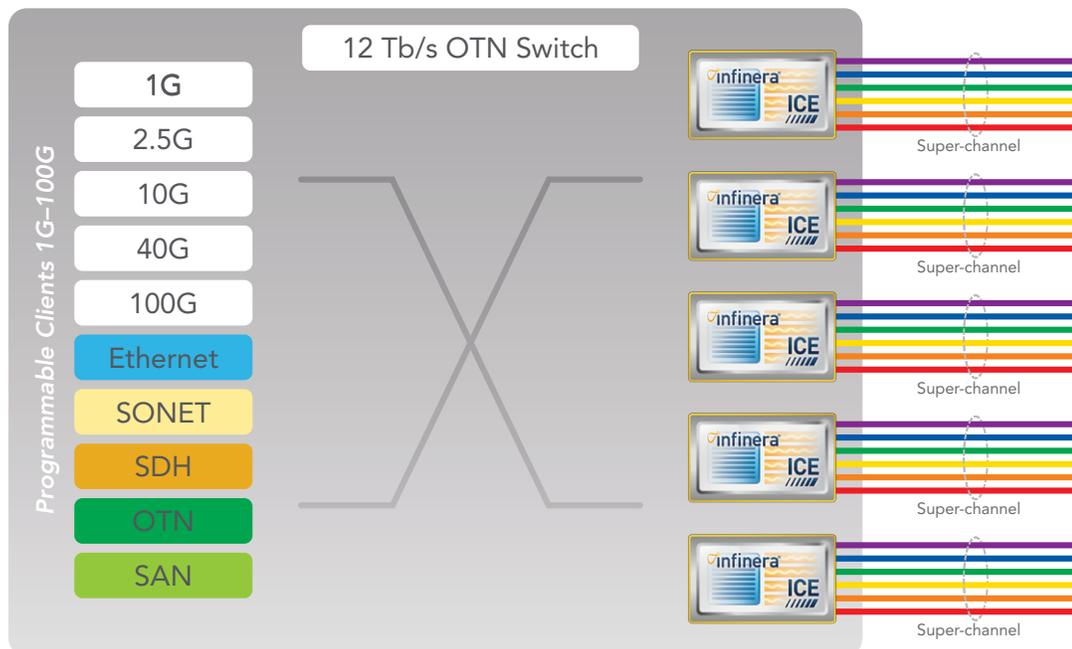
Figure 5: XTC Series: OTN Switching with ICE
