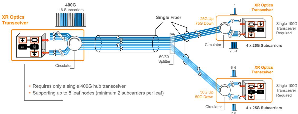
Figure 3: XR optics operation over single-fiber working infrastructure
