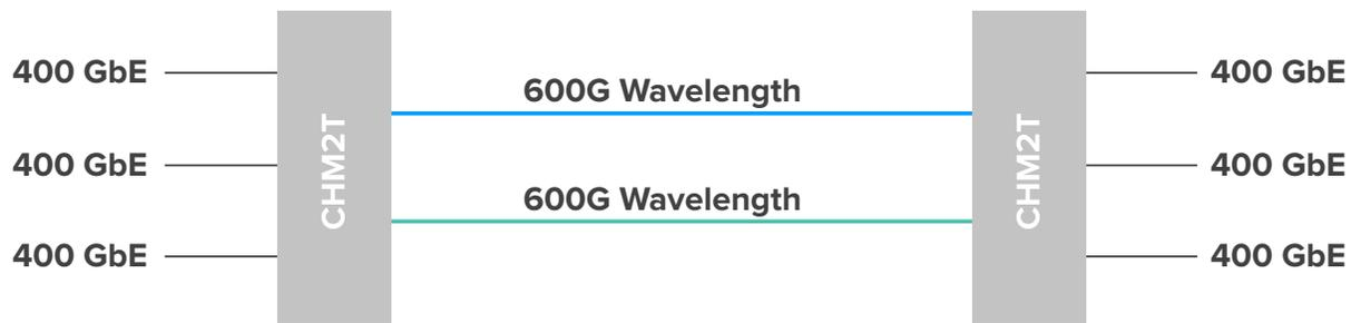
Figure 3: 3 x 400 GbE over 2 x 600G wavelengths – 33% cost savings
