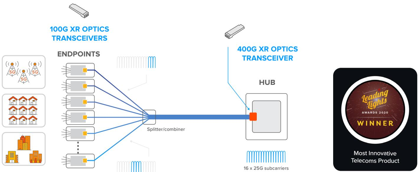
Figure 1: Direct low-speed to high-speed optical interconnectivity with XR optics
