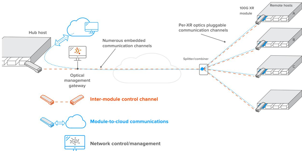
Figure 2: XR Optics flexible end-to-end management
