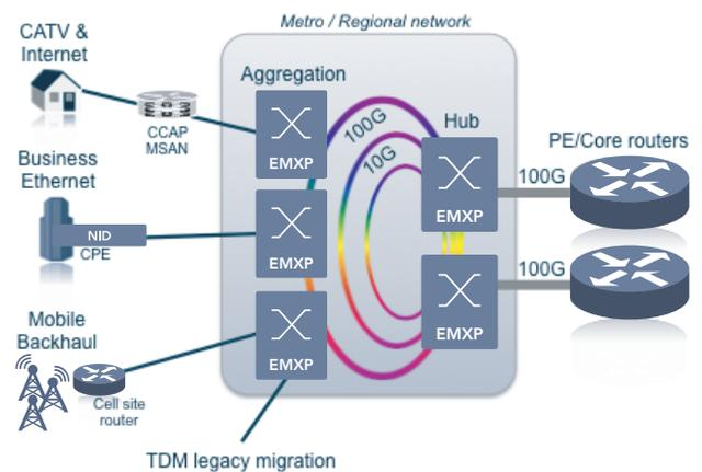
Fig 2. PT-Fabric in a Network Scenario with other EMXP Packet-Optical Transport Switches.
