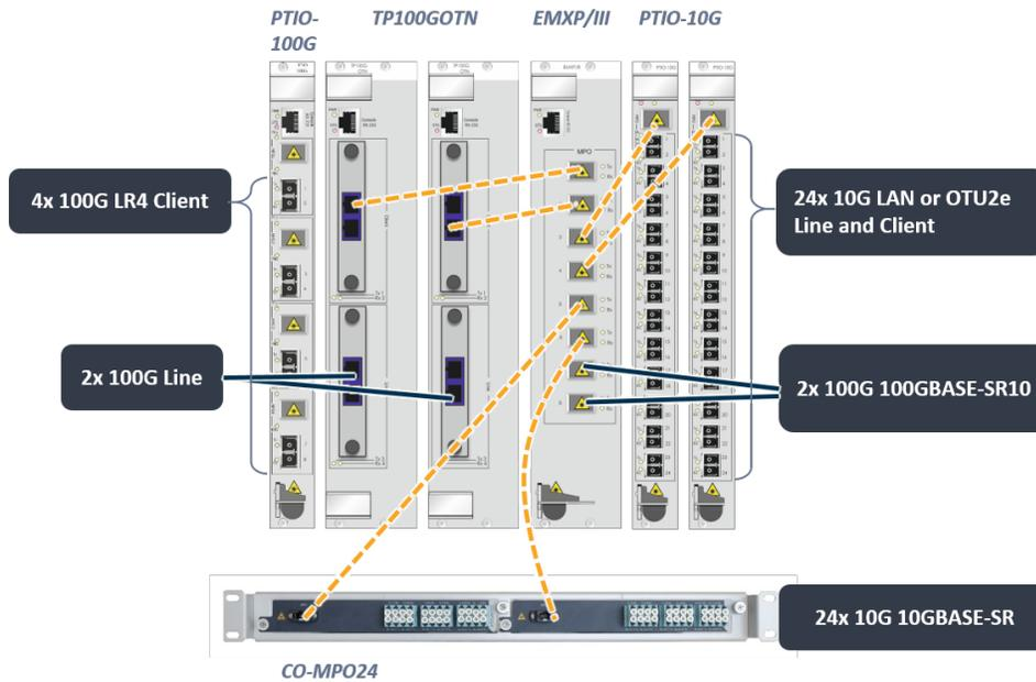
**Fig 1.** PT-Fabric Providing Multiple 10G and 100G Services using the 100G Transponder, PTIO-100G and PTIO-10G Interface Modules and the XTM Series-based CO-MPO24 Multimode Break-out Box.
