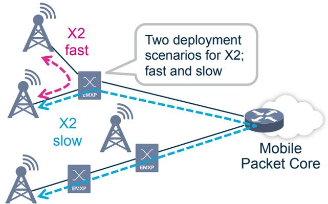
Fig 2. Low Latency in the Mobile Backhaul Solution Makes It Ideal for Transporting X2 Signaling Used in LTE Networks.
