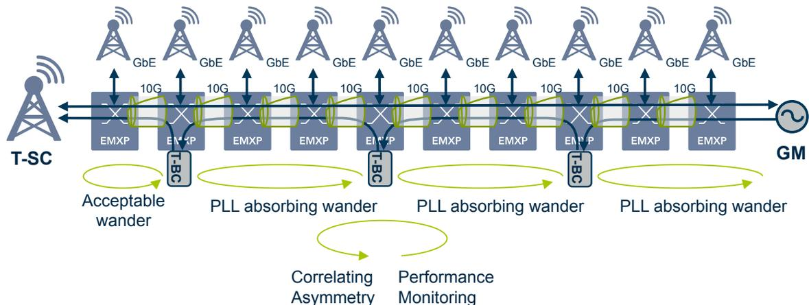
**Fig 6.** The Infinera T-BC Implementation Reduces Wander Significantly.
