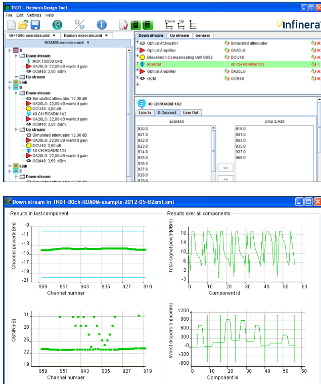
Fig 1. Two Screenshots from TNDD Showing the Optical Performance of an 80-channel ROADM Example.
