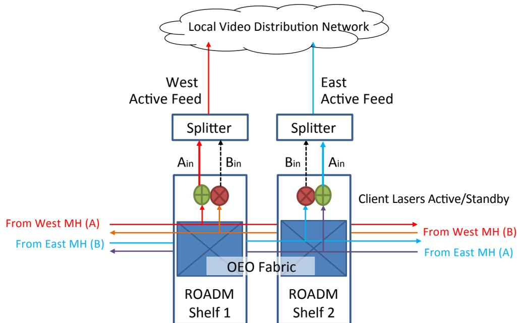
Figure 3—V2B 2.0 Typical Market DWDM Transport Detail
