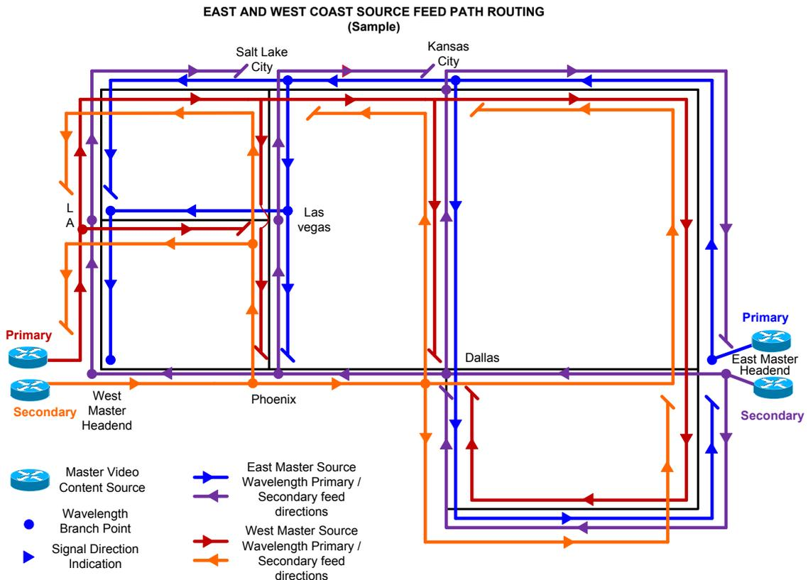
Figure 2—V2B 2.0 General Wavelength Multicast Tree and Branch Topology
