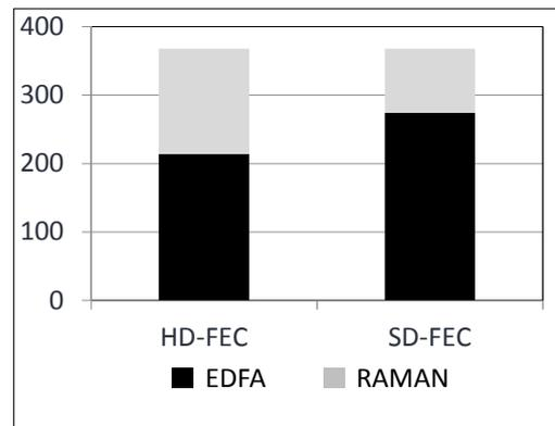
**Fig. 6:** Types of line amplifiers deployed with HD-FEC vs. SD-FEC
