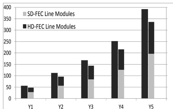
Fig. 4: Total Number of Line Modules deployed over a period of 5 years with HD-FEC vs. SD-FEC. With only HD-FEC line modules, 56 line
