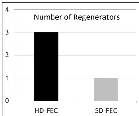
**Fig. 5:** Average number of regenerators deployed with HD-FEC vs. SD-FEC
