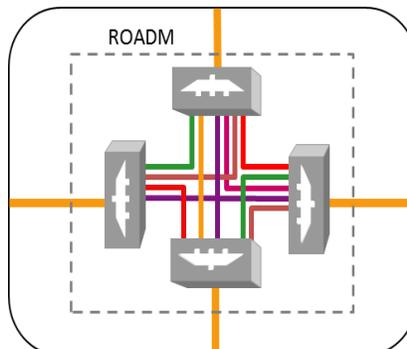
Fig. 1(b) Optical Switching Architecture
