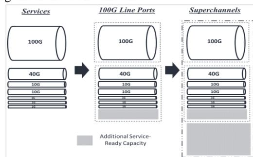
Figure 4 Grooming of Client Services in Super-Channels
