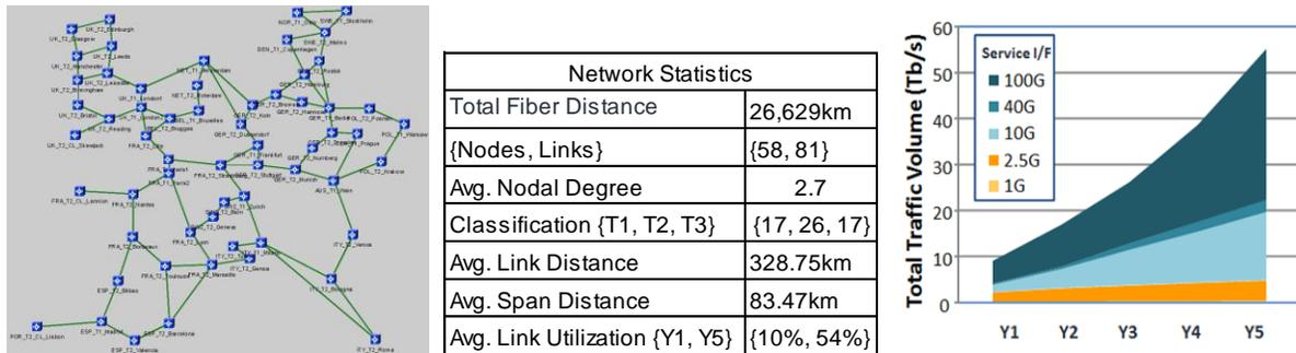
Figure 2 Pan European Network Model Specifications
