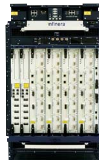
The Infinera DTN platform's use of pluggable tributary adapter modules allows high-density digital add/drop of multiple services. The DTC chassis accommodates 23-inch and ETSI racks.
