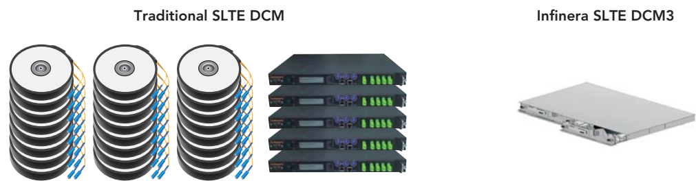
Figure 3: Traditional SLTE dispersion compensation can require up to 20 times the space of the Infinera DCM3 solution.
